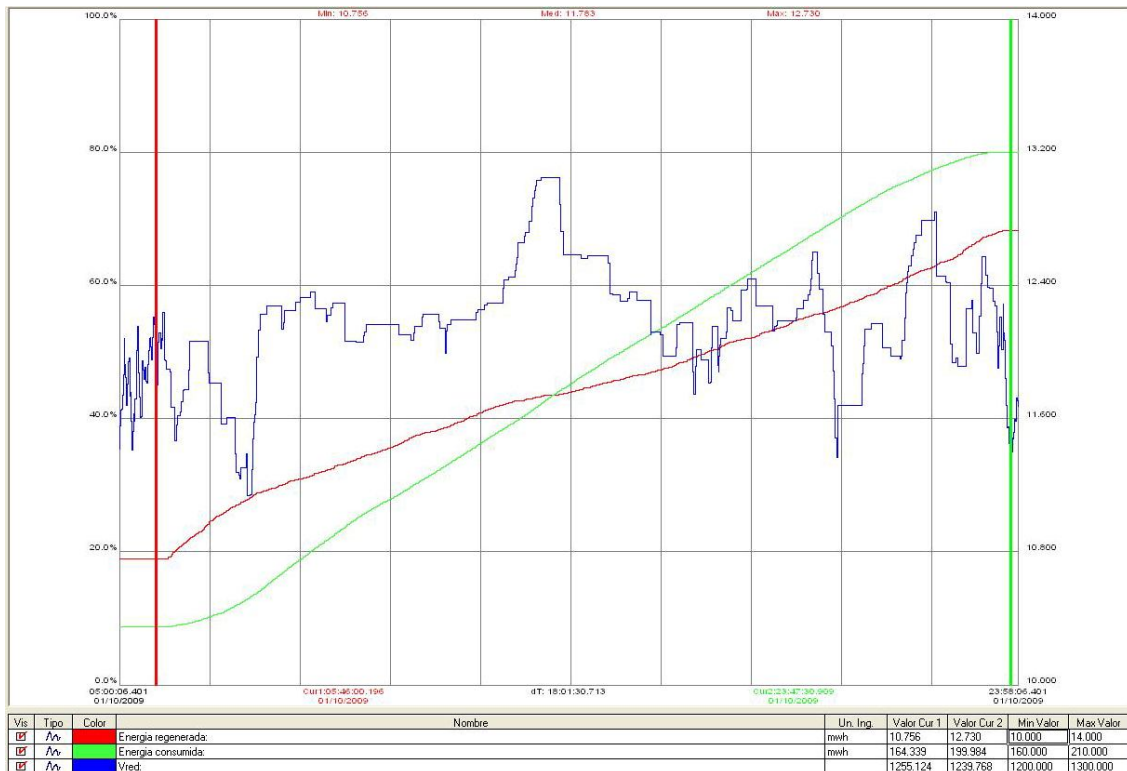
Figure 5: Evolution of energy consumed, energy recovered and grid voltage.
