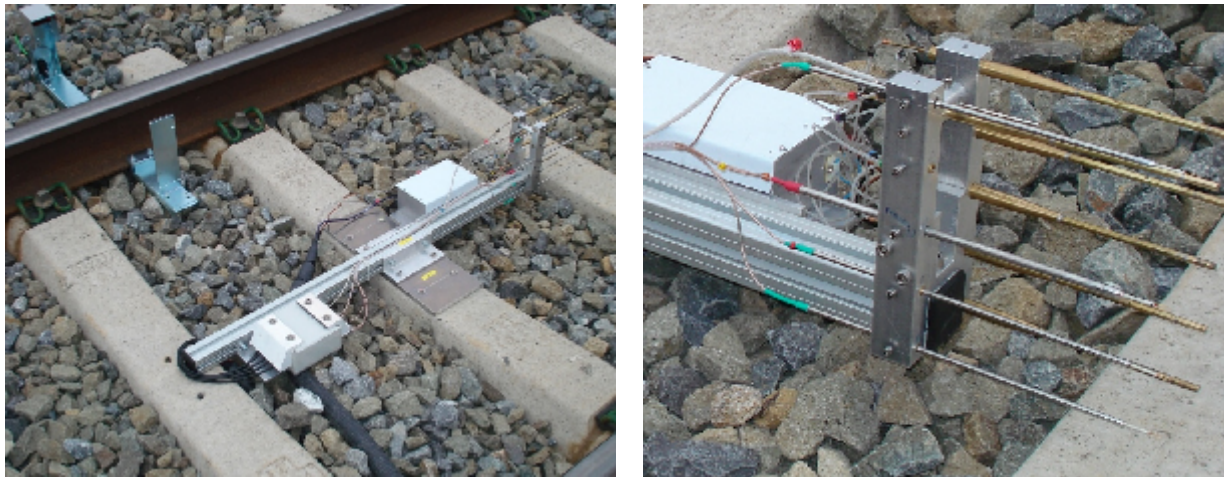
Figure 5: Installed Pitot-static and hot-film rakes. Left: general view showing also the infrared train position sensor. Right: detailed view of the probes.
