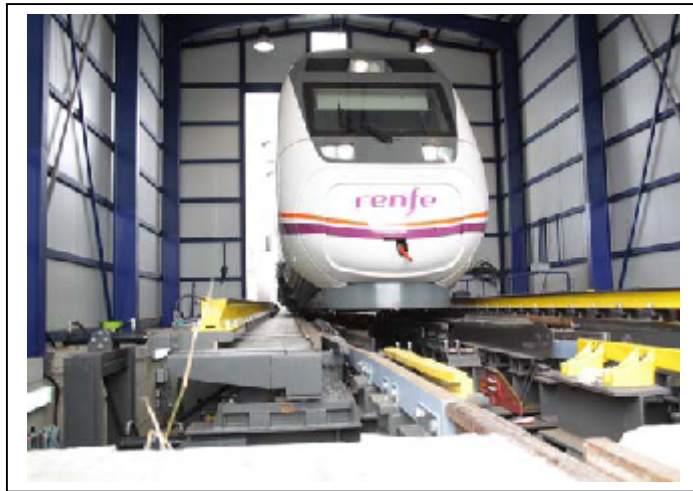
Figure 8. CAF train passing over the new TCSR3 platform
