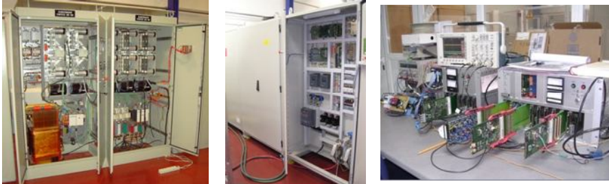
Figure 2. Power electronics converters (machine-side, grid-side and catenary converter) and control platform at the laboratory tests.
