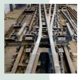
Slip Crossings for ADIF, the supply of all turnout systems to Line 2 Metro de Santo Domingo (Dominican Republic), or different R+D+I samples to be applied at the lockers for double gauge turnouts, or at the swing nose crossings for the Spanish High Speed Turnout family "AV4" from ADIF.
