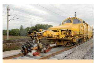
mated welding robot with the new closure welding technology has already been approved by several European Rail Authorities. Plasser & Theurer will expose this innovation at Innotrans reminding that we are the leading company in construction, maintenance and renewal technology of railway superstructures.
